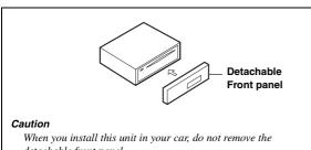
When you install this unit in your car, do not remove the detachable front panel. If the detachable front panel is removed during installation, you might press too hard and warp the metal plate that holds it in place.
