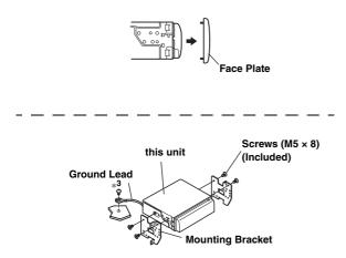
Secure the ground lead of the unit to a clean metal spot using a screw (\*<sup>3</sup>) already attached to the vehicle's chassis.
