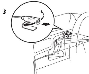
Secure the microphone cord using cord cramps (not supplied) if necessary.
