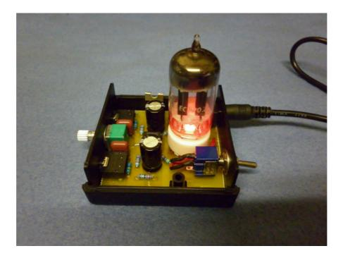
Finally positioned in a Hammond case With JRC4556 in place Needs a 12volt 1 amp Regulated DC supply
