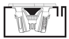
Box is given as internal air volume including driver displacement
