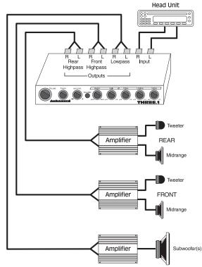
Figure 6: THREE.1 with source unit and three amplifiers
