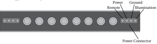
Figure 5: Rear View of the THREE.1
