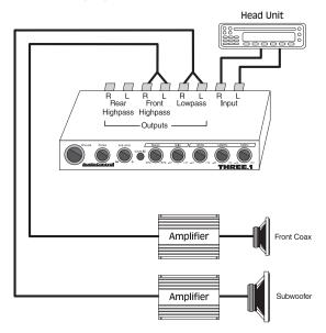
Figure 9: THREE.1 with source, front amp, and sub amp
