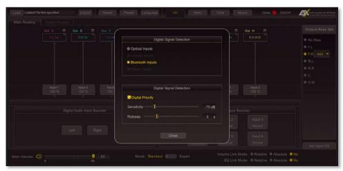
The digital inputs can be prioritized so that they are switched over when a signal is received. Here Bluetooth gets priority; after 5 seconds of silence, it will be switched back to analog
