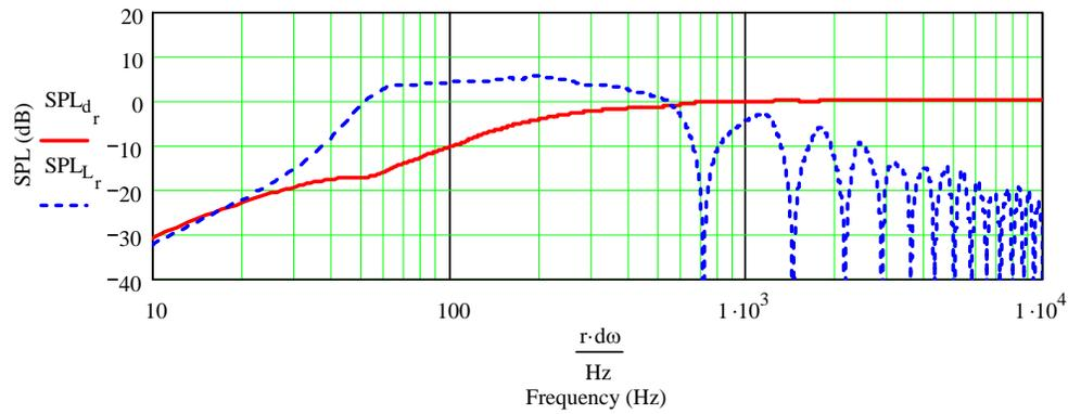
Figure 7.20 : Back Loaded Exponential Horn Response – Baseline Configuration with a Coupling Chamber, Driver Position Ratio  $\xi = 0.5$ , and Fiber Damping
