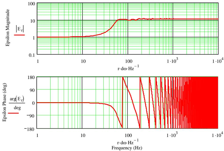
Figure 7.16 : Back Loaded Exponential Horn Response – Baseline Configuration with a Coupling Chamber and a Driver Position Ratio  $\xi = 0.0$
