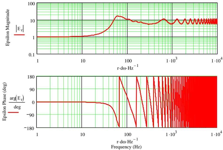
Figure 7.14 : Back Loaded Exponential Horn Response – Baseline Configuration with a Coupling Chamber and a Driver Position Ratio  $\xi = 0.5$
