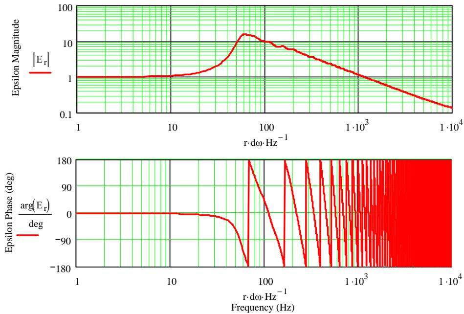
Figure 7.10 : Back Loaded Exponential Horn Response – Baseline Configuration with a Coupling Chamber
