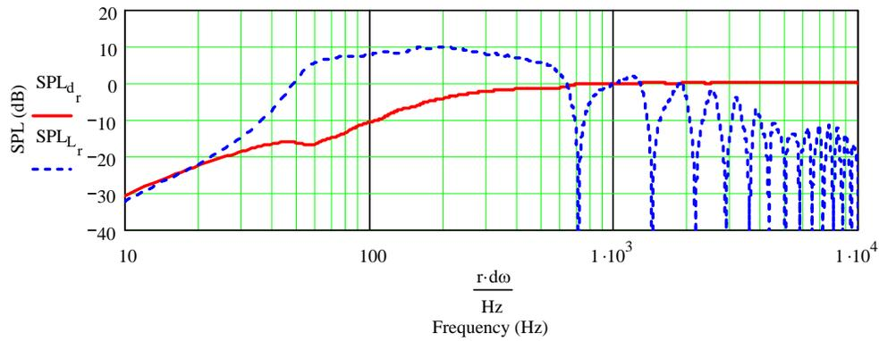
Figure 7.17 : Back Loaded Exponential Horn Response – Baseline Configuration with a Coupling Chamber and a Driver Position Ratio  $\xi = 0.5$
