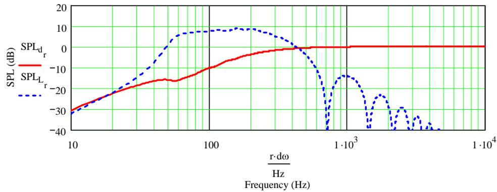
Figure 7.11 : Back Loaded Exponential Horn Response - Baseline Configuration with a Coupling Chamber
