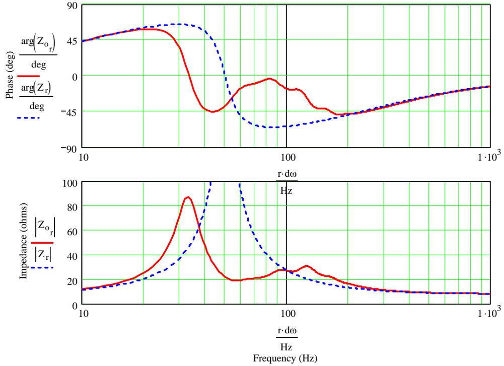
Figure 7.12 : Back Loaded Exponential Horn Response - Baseline Configuration with a Coupling Chamber
