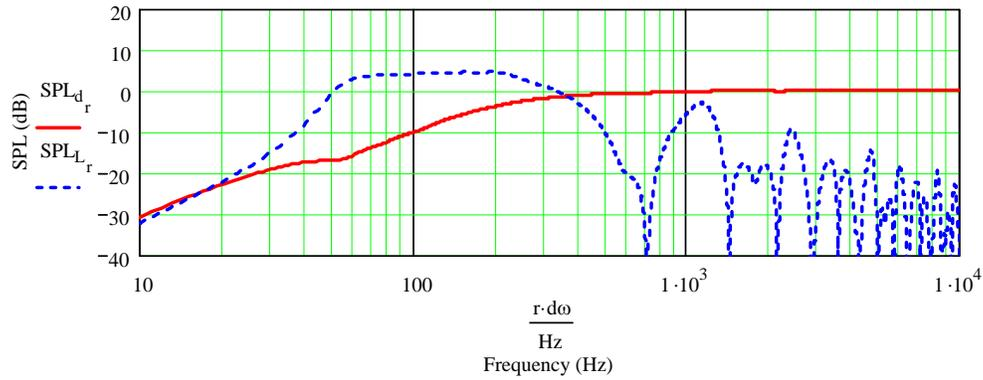
Figure 7.21 : Back Loaded Exponential Horn Response – Baseline Configuration with a Coupling Chamber, Driver Position Ratio  $\xi = 1.0$ , and Fiber Damping
