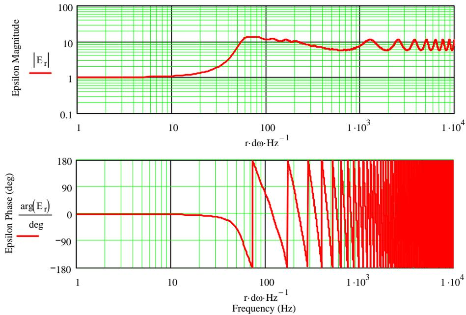
Figure 7.15 : Back Loaded Exponential Horn Response – Baseline Configuration with a Coupling Chamber and a Driver Position Ratio  $\xi = 1.0$
