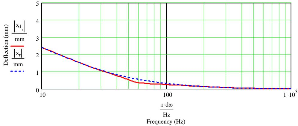
Figure 7.13 : Back Loaded Exponential Horn Response - Baseline Configuration with a Coupling Chamber
