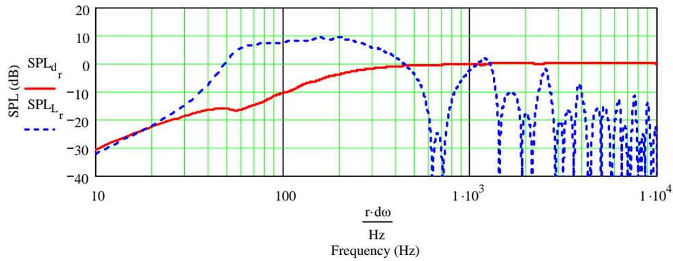
Figure 7.18 : Back Loaded Exponential Horn Response – Baseline Configuration with a Coupling Chamber and a Driver Position Ratio  $\xi = 1.0$
