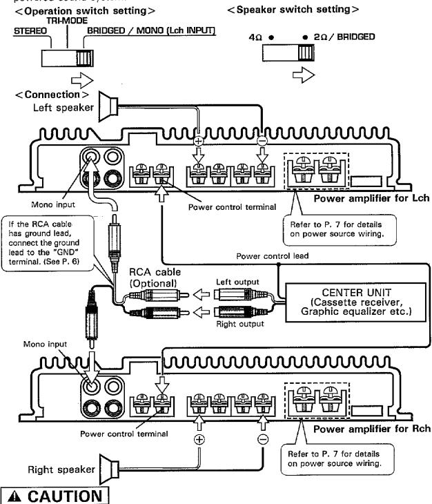
Be sure that the combined impedance of your speaker system as seen from the KAC-923/823 is at least 2 ohms. An impedance of less than 2 ohms will damage the amplifier.
