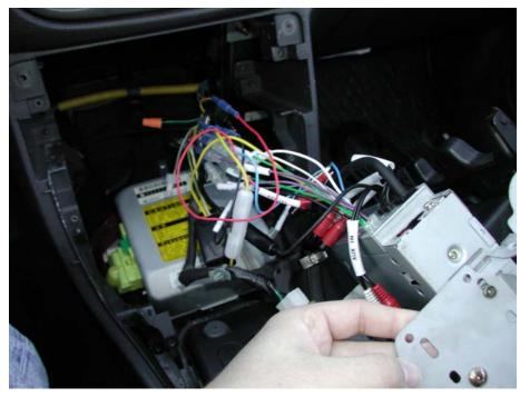
Here is the stereo pulled out. The box with the big yellow sticker on it is the airbag control box, leave it alone! Now you can disconnect your current stereo and connect up your new one. Below I have included the pin-out for the 14-pin connector standard in a Subaru. This information was obtained from this Usenet Post:
