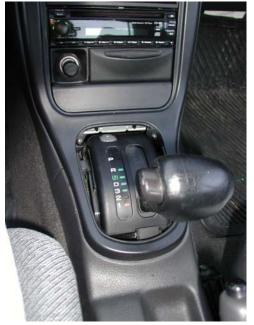
Now, open the cup holder. We are then going to remove the screws to the left and right of the cup holder. This frees the top portion of the outer trim assembly for the center of the dash.
