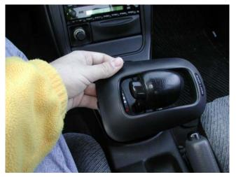
The next step is to remove the shifter cover. To do this note the small notch at the bottom, near the parking brake, insert a regular screwdriver there to pop it up and then rotate it 90 degrees to take it over the shifter. The picture on the left shows this process com-
