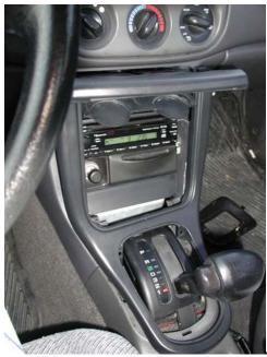
The next step is to remove the outer dash trim piece. To do this just start pulling up at the top and work your way down. I have shown the before and after pictures on the left and right respectively.
