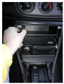
Pull the center dash rack out about 4 to 6 inches. Once you have done this, reach over to the right side and pull off the ground connector as shown in the picture on the right. Continue to pull the rack out. This step is why it is important to put the car in a gear lower than park. You will find that if you do not, you won't be able to pull the rack out. The shifter will get in your way which is very annoying when your hands are busy with other things.
