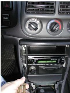
Now, remove the four screws holding in the center dash rack. This rack holds the entirely CD, ashtray, lighter, etc assembly. Be careful, underneath this unit is the airbag control system. We would not want to inadvertently damage it in the process. On the next page is a large picture showing the four screws to remove. The picture on the let is before removing them. On the right is after.
