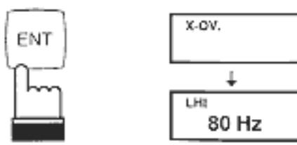
Press the ENT (Enter) button on the Remote Controller to activate the  $\blacktriangleright\blacktriangleleft$ ,  $\blacktriangleup$  and  $\blacktriangledown$  buttons. The display shows the channel and frequency for 5 seconds.
