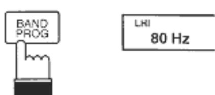
Press the BAND/PROG button on the Remote Controller to select the frequency range to be adjusted while the channel and frequency are displayed.
